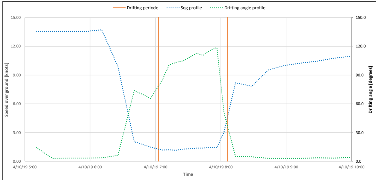
Figure 7-18 Average speed and drift angle profile of cargo vessel (158m)
