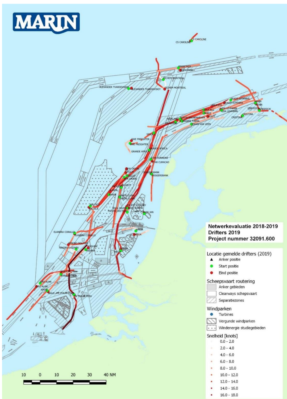
Figure 7-1 AIS-tracks including speed of ground during reported drifting incidents in 2019 (Jan – August)
