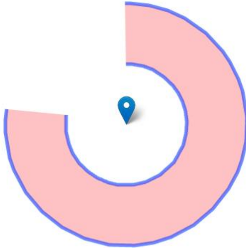
Figure 2.1 Donut-shaped area which was used to calculate the MTR from the horizontal radar data in the Luchterduinen Wind Farm. The blue marker shows the radar position. The white triangle represents the blanking area of the radar to avoid radiation from the turbine on which the radar is installed.
