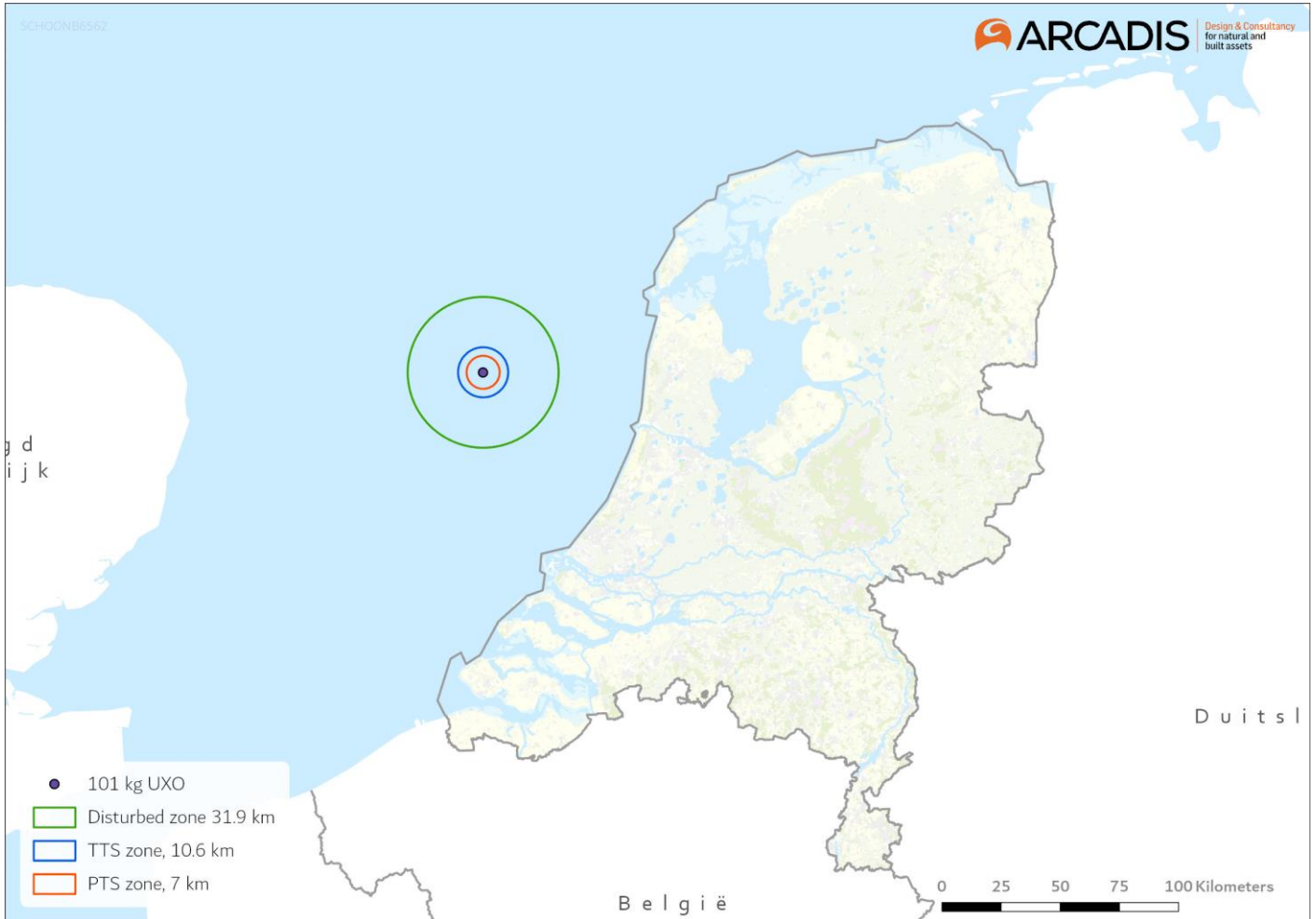
Figure 16 Surface areas in which harbour porpoise behavioural response (green), TTS (blue) and PTS (red) occurs for a single UXO clearance with a net explosive quantity of 101 kg, which is equal to the most found aerial bomb.
