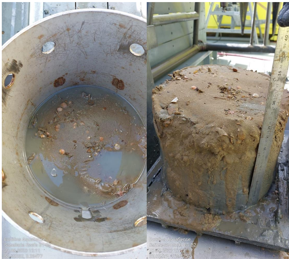
Figure 4.2: Type A sample (location B1-B2), containing some empty Sabellaria tubes, a sandy top layer and a silty sublayer.
