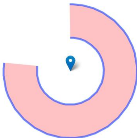
Figure 2.1 Donut-shaped area which was used to calculate the MTR from the horizontal radar data in Luchterduinen wind farm. The blue marker shows the radar position. The missing part of the donut the represents the blanking area of the radar to avoid excessive reflection from the turbine on which the radar is installed.
