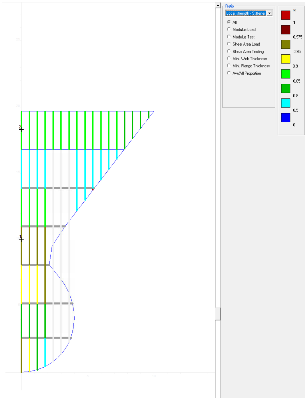
Figure 52 – Transverse Bulkhead Fore – Local Strength Check – Stiffeners
