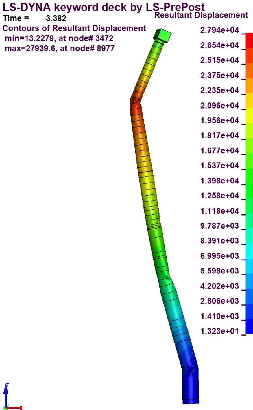
Figure 117. Resultant Displacement Foundation Tower [mm]
