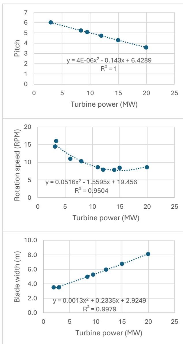
Figure III.7.1 Graphs underlying the extrapolations. From top to bottom: pitch, rotation speed and blade width
