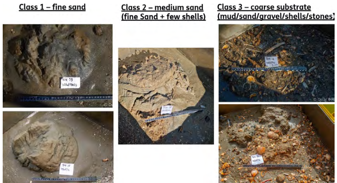
Figure 3.6: Box core samples showing the sediment corresponding with the three classes of fine sand, medium sand and coarse substrate.
