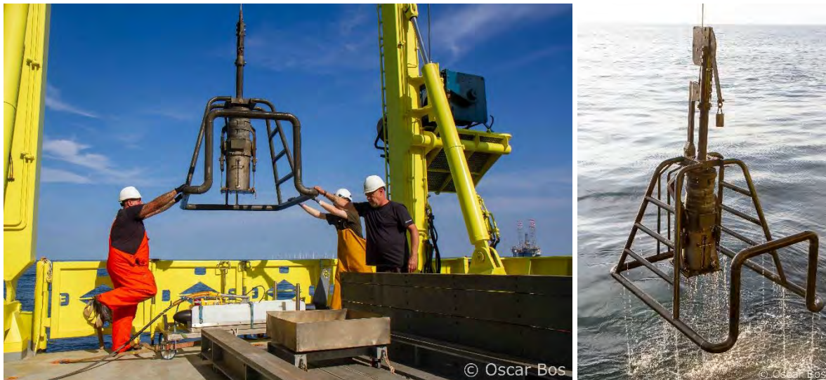
Figure 12. The Rijkswaterstaat box corer (0.315 m diameter, surface 0.078 m 2 ) (photo: Oscar Bos).
