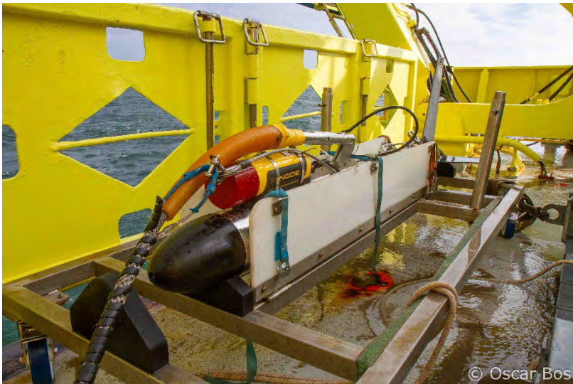
Figure 5. Side scan sonar towed fish with the USBL, which was deployed during each night.
