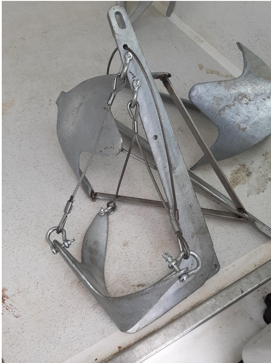
Figure 19 Variant 4 with three steel cables.
