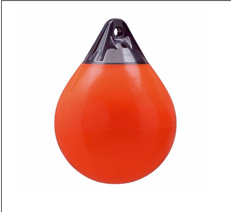
Figure 13 Polyform A1 buoy, buoyancy 7.8-13 kg, weight: 1.15 kg. Length: 38.0 cm. Diameter 29.5 cm.
