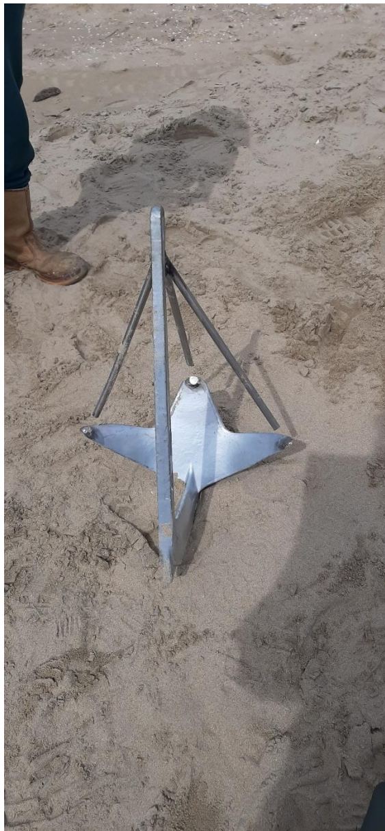
Figure 18 Variant 3 with cut through bars.
