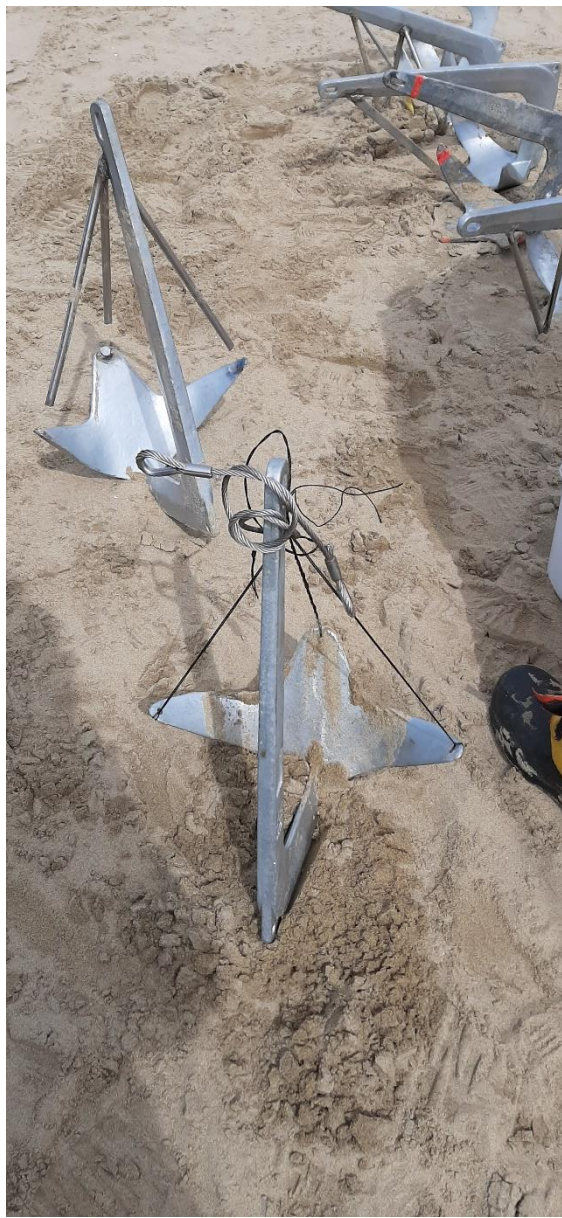
Figure 20 Variant 5 with three thin ropes cables.
