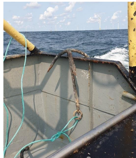
Figure A1.3: 29/08/2023 light dredge anchor used for recovery of string without markings
